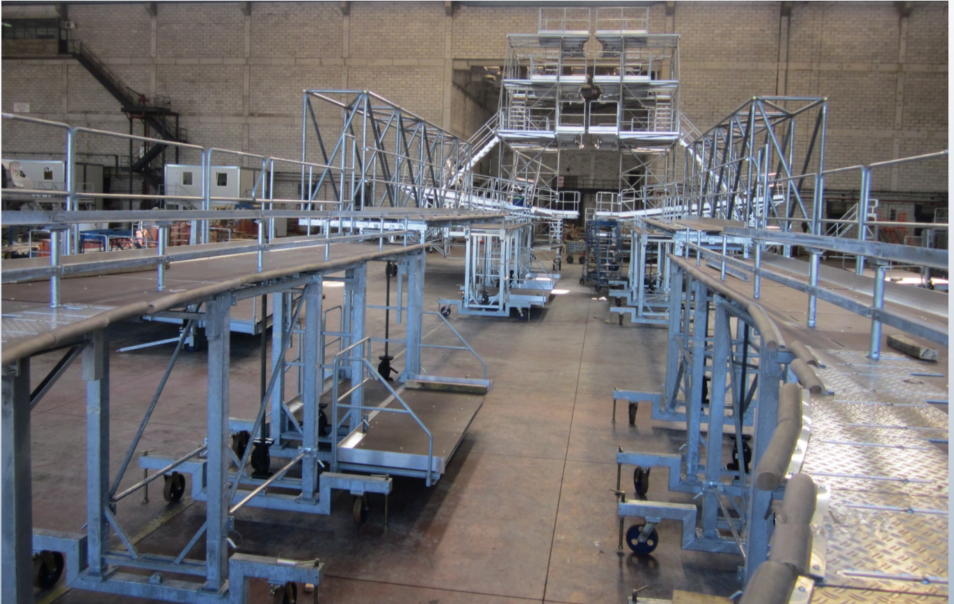
Narrowbody Docking System for Maintenance Works on Various Aircraft.
